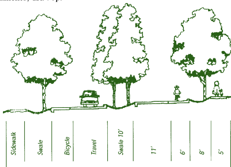
Incorporate stormwater treatment into street design by adding trees and swales. From Green Neighborhoods, a publication of NeighborhoodLAB, http://neighborhood.uoregon.edu/ .
